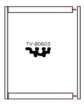
Pack out the glass on the opposite side to the slim interlock in order for the glass to be pushed into the bonding agent correctly.
