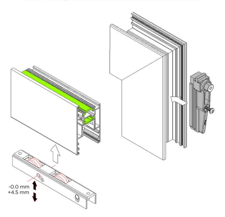
Place wheels approx 100mm from the edge of the profile, with the adjuster screw pointing to the outside.
