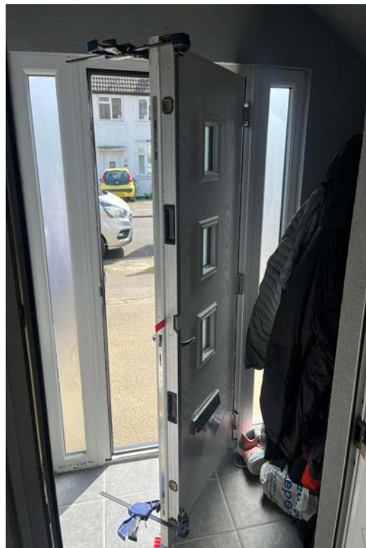
2. Straight edge on the concave side, from a distance. Packer to show bow
