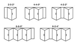
\*No external access as standard for these configurations Handles displayed are internal positioned
