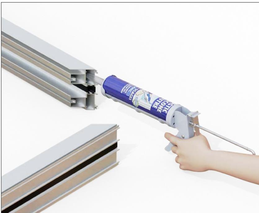
It is important to seal the bottom profile at both ends to prevent water from draining into the cleats.
