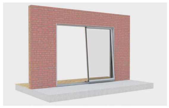
Swing bottom of sash above running gear.
